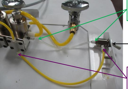
Connect constant air to the barb farthest away from the toggle (input) on the master on/off valve.
